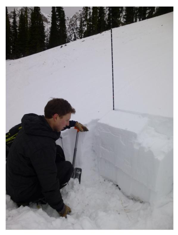
This pit was dug on a wind loaded slope with small facets under the wind slab. It broke clean in our stability tests. Luckily this instibility is not found in most areas, but it's worth searching for. ECTP18. Photo: GNFAC
