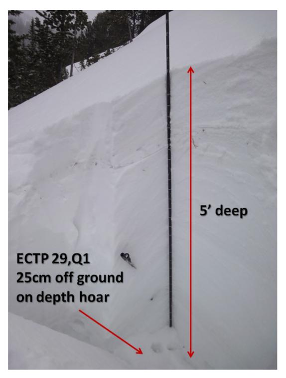
This pit was dug on a north facing slope at Lionhead. The ECT failed on 29 taps on large depth hoar crystas less than a foot off the ground. Although it would be difficult to trigger when it is this far under the surface, in areas wher the snowpack is thinner a snowmobiler could initiate a fracture that would propagate to deeper slopes like this one. Photo: GNFAC
