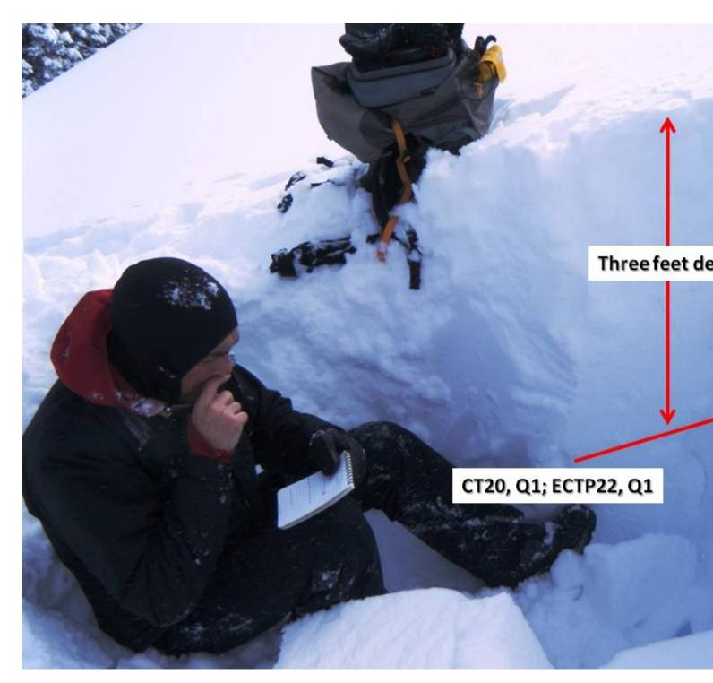
I found the layer of small-grained facets breaking and propagating in one of my snowpits. I was surprised by this since we were not finding it on other slopes. Even though this instability is isolated, its worth looking for. Photo: Jordy Hendrikx
