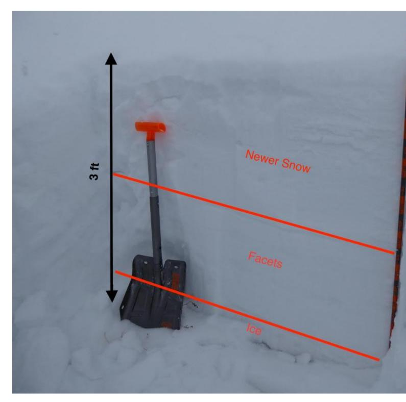
A north facing snow profile near Daisy Pass in Cooke City. There is an ice layer on the ground. Above the ice, half the snowpack is faceted October snow and half is November snow. No propagation in an Extended Column Test. Photo: GNFAC
